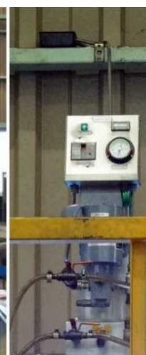
300 ton press hydraulic oil ↑ Miracle Boy SRC-811-8V connected to the tank On the stage so as not to block the space around the press
