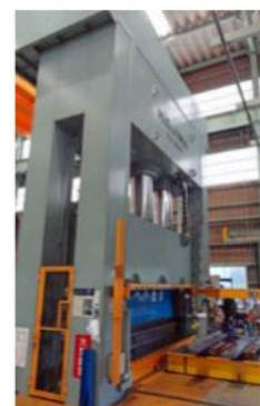
300 ton press hydraulic oil ↑ Miracle Boy SRC-811-8V connected to the tank On the stage so as not to block the space around the press
