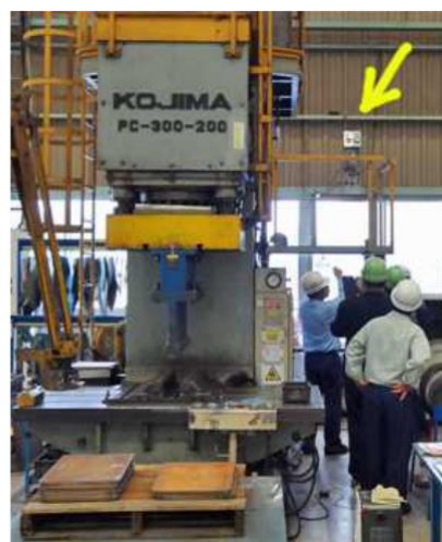
300 ton press hydraulic oil ↑ Miracle Boy SRC-811-8V connected to the tank On the stage so as not to block the space around the press
