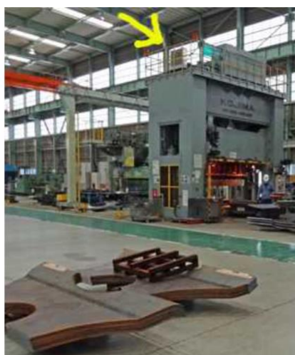
Miracle Boy SRC-812-6V connected to a 1500 liter hydraulic oil tank of a 1000 ton press
